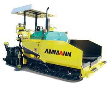
Tracked machine with rubber pads; automatic tensioning device system with grease accumulator. Hydrostatic transmission with two variable flow rate pumps which feed two motors with two displacements directly fastened to the planetary gearboxes which operate the tracks. Mounted on each pump, an electronic and proportional control gives a progressive start and stop,
